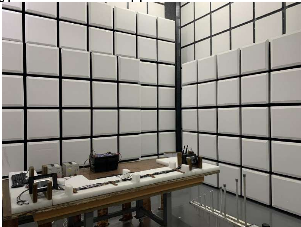
Log-periodic Antenna test set up photo in the anechoic chamber
